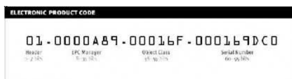
Figur 3: EPC - Electronic Product Code
